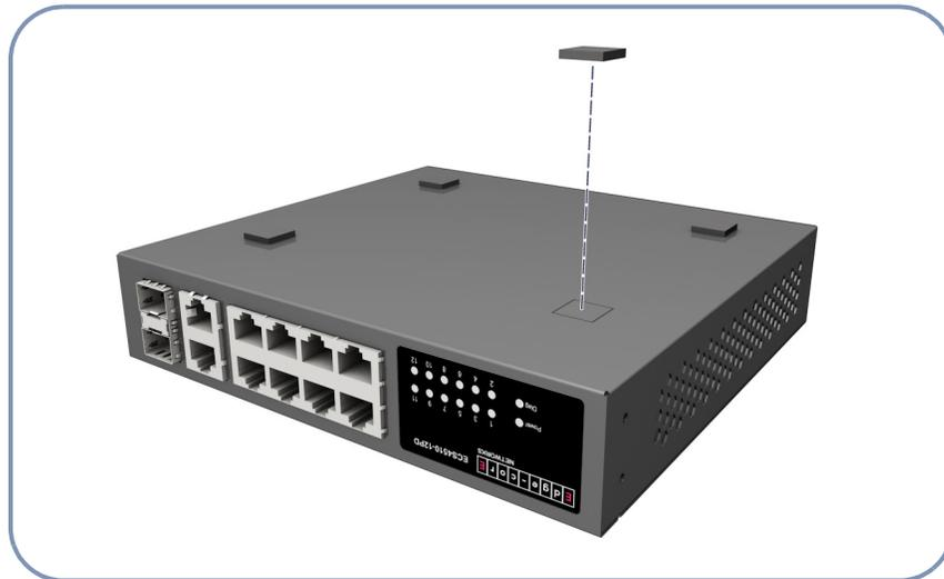
2. Set the device on a flat surface near an AC power source, making sure there are at least two inches of space on all sides for proper airflow.
