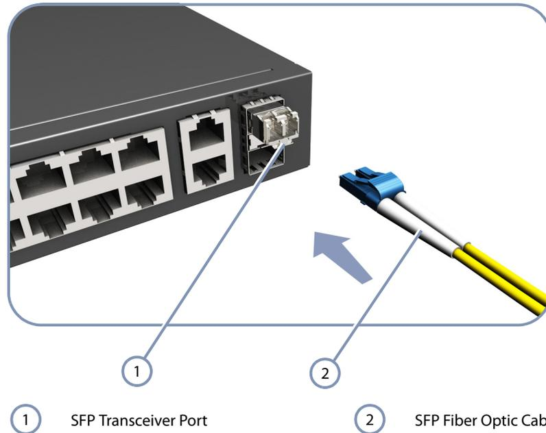
4. As a connection is made, check the Link LED on the switch to be sure that the connection is valid.
